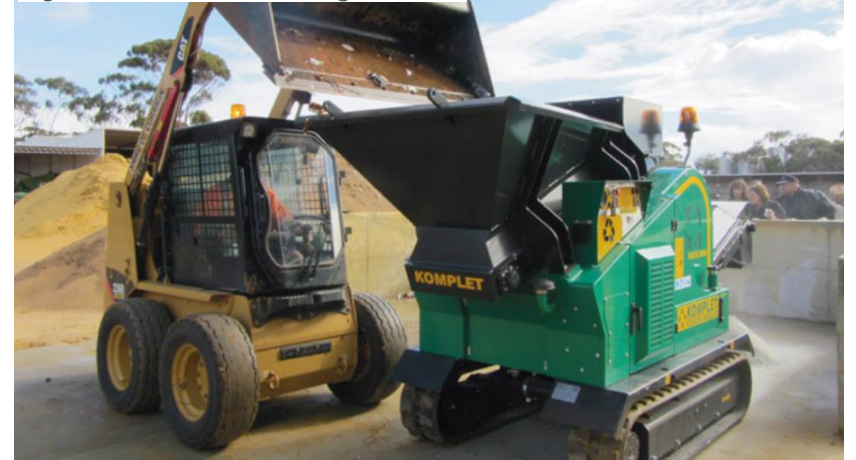
Figure 27 – Glass crushing machine
